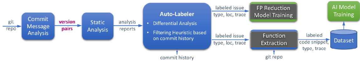
Figure 3.1: A schematic of the D2A generation pipeline. This figure was taken from [94].
