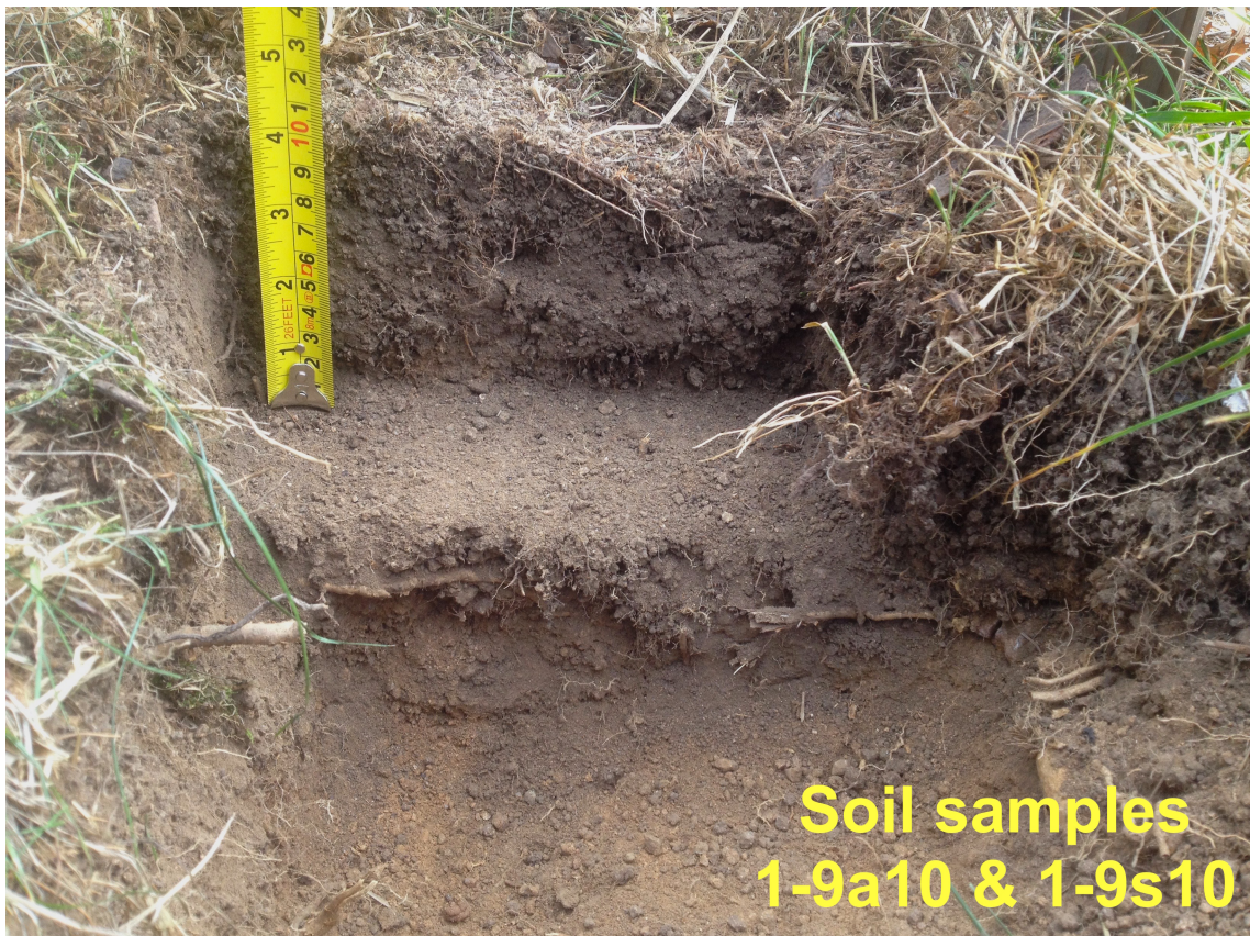
Figure 7 Typical preparations for soil sample collection at 10 cm depth. Sample ID clarification (exemplary case 1-9a10 and 1-9s10): first number stands for sampling period (1 – autumn), second number denotes subplot (9), the letters a and s are for sampling point and mixed sample identification respectively and the third letter (10) marks the depth of sampling. Note how dry the soil profiles were during the first sampling
