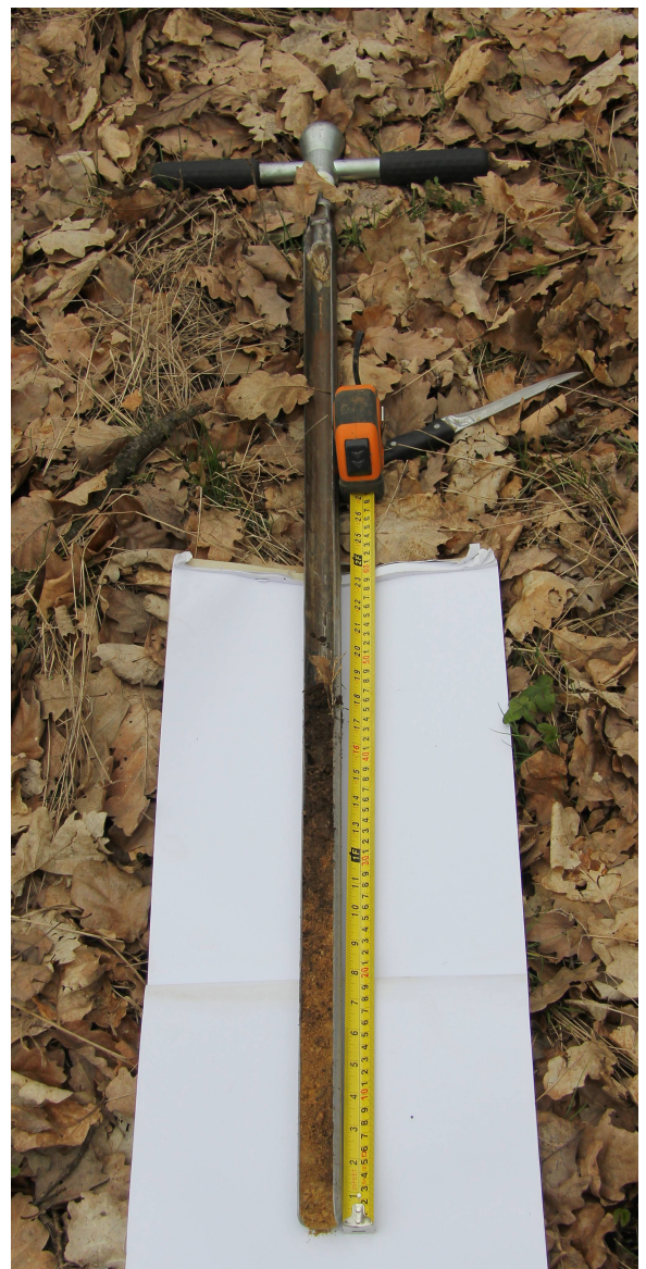
Figure 8 An example of hammerhead soil probe and recovered sample.
