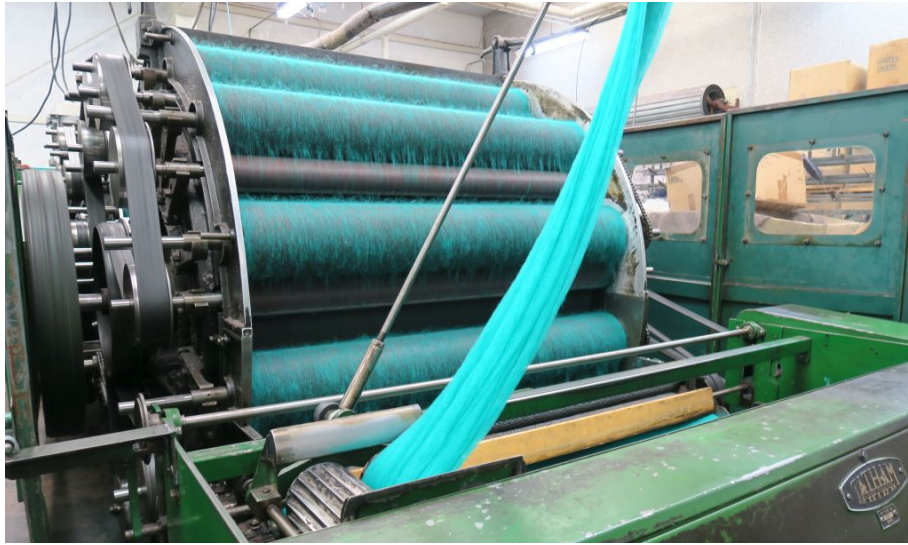
Figure 1.2: Carding machine straightening colored wool. This is an industrial machine, the laboratory uses much smaller one. [15]
