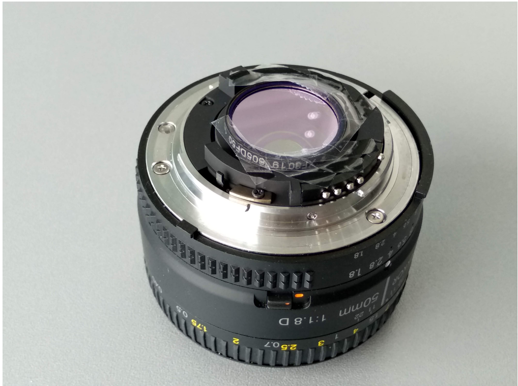
Figure A.7: Light filter temporarily fixed to the back side of a lens. Note professional attachment.
