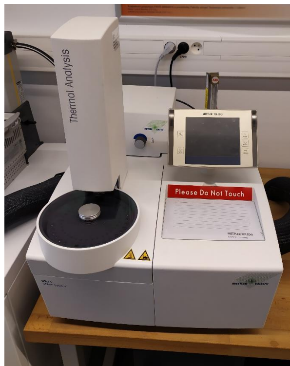
Obr. 3.4 DSC kalorimetr Mettler Toledo DSC 1/700
