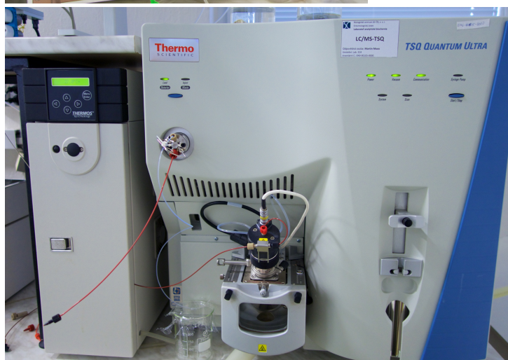
Fig 9: UHPLC-Triple Quadrupole System used in this study (laboratory BC-CAS)
