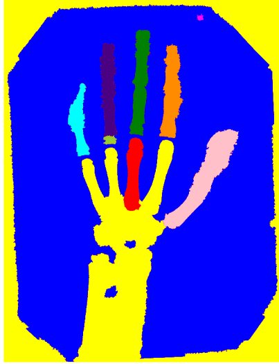
Figure 2.14: Watershed image segmentation output. Image shows the result of watershed segmentation on one of the X-ray database image. Many inaccuracies can be observed in this method output.
