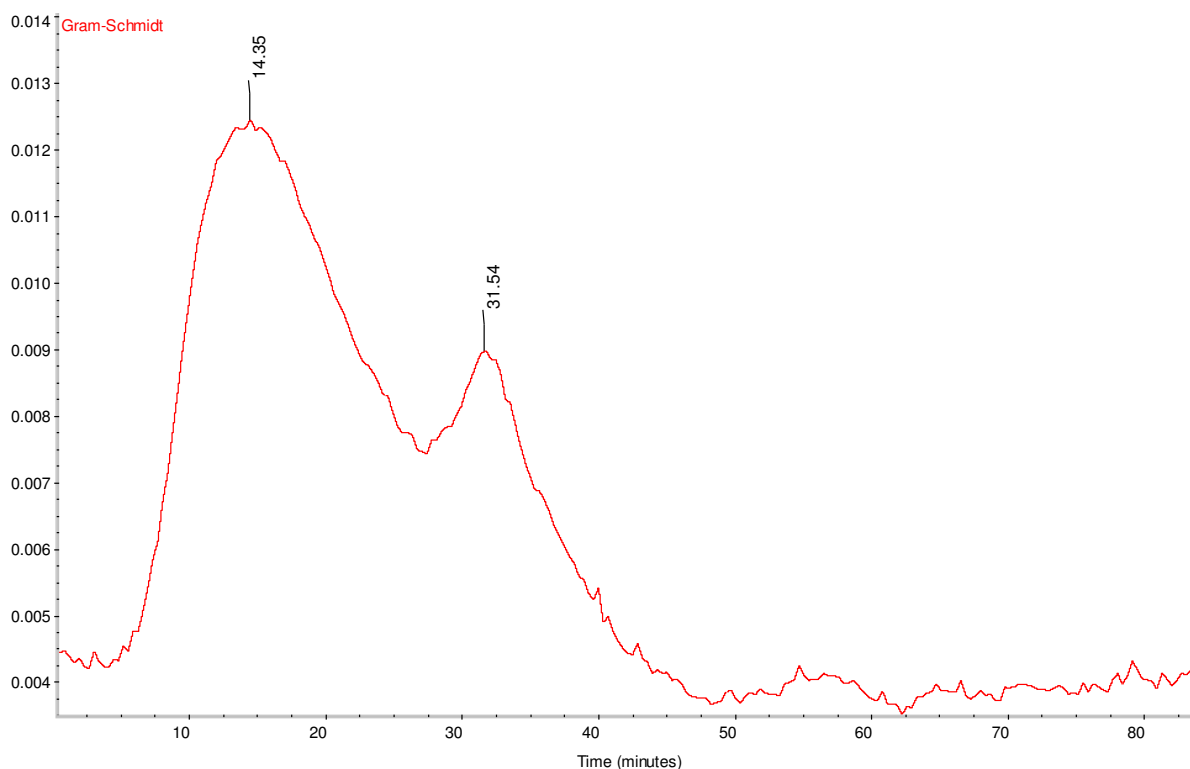
Fig. 27 Gram-Schmidt analysis of hydrolysed TIETH R = 4
