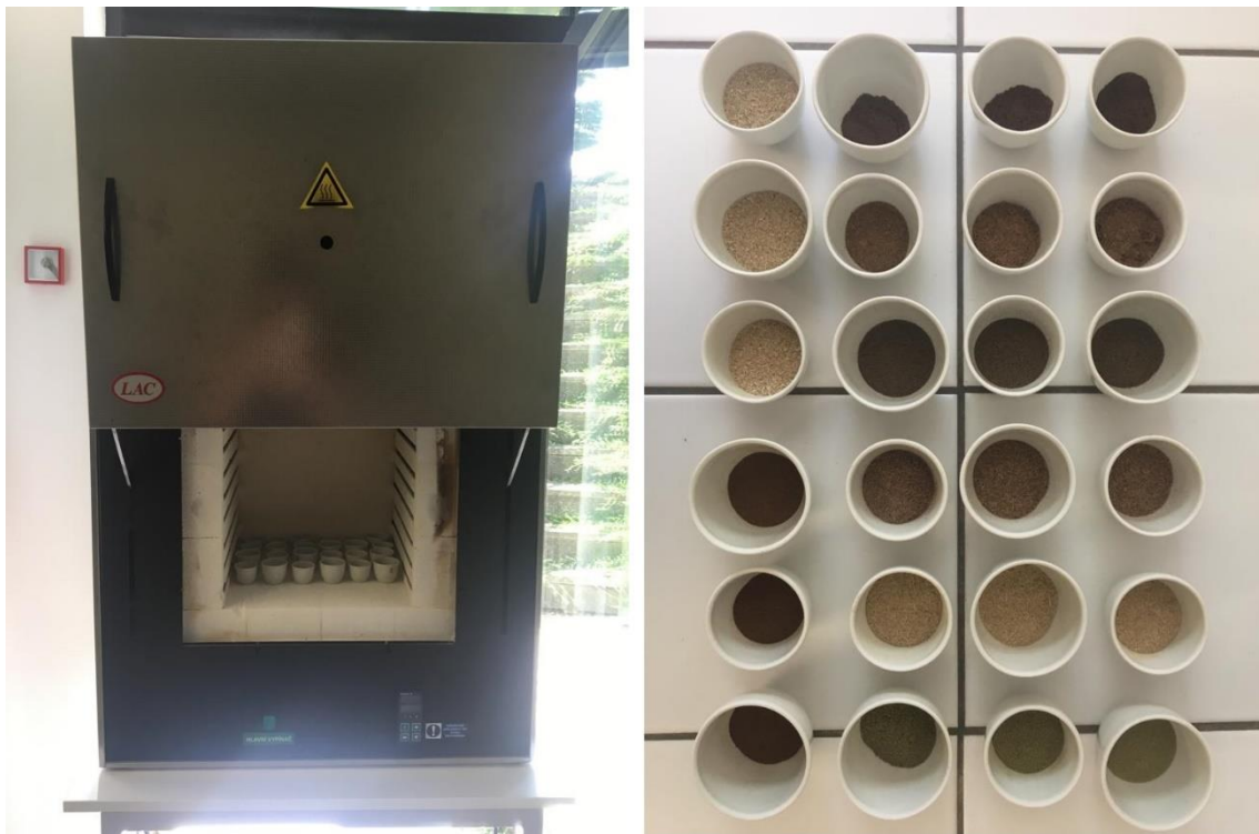
Figure 22: The dry basis samples tested in the ash content test equipment, LAC
