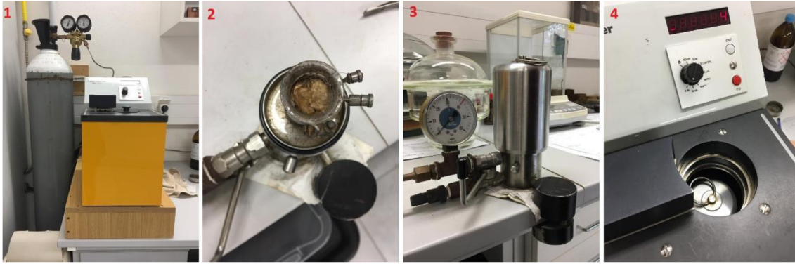
Figure 23: The experimental setup of the calorimeter for the CV determination
