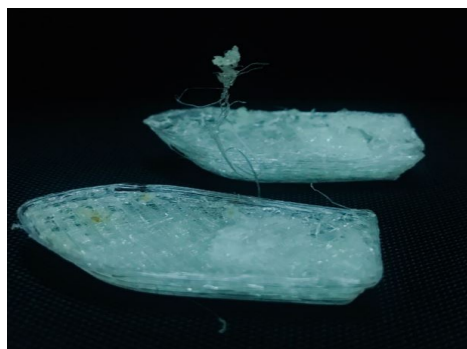
Figure 29 Defects in the Printed parts in PVA
