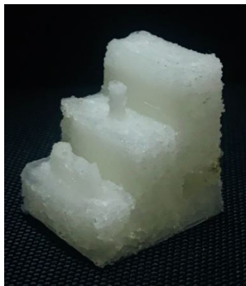
Figure 32 Newly printed part with thickness of 0.25mm in PVA
