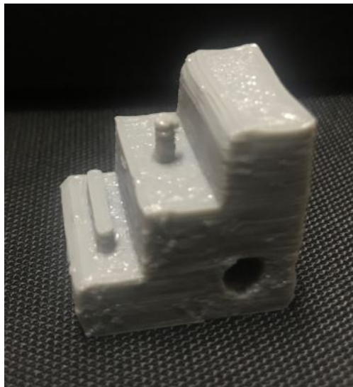
Figure 24 Newly printed part with thickness of 0.3 mm in PLA
