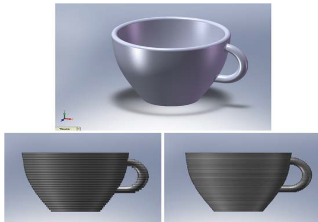
Figure 1 Cup printed with different layer thickness [1].
