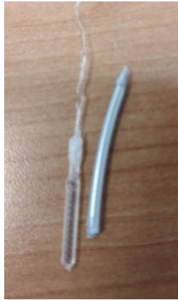
Figure 31 Material elongation of PVA in the printer
