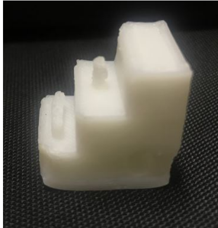
Figure 38 Newly printed part with thickness of 0.3 mm in HIPS
