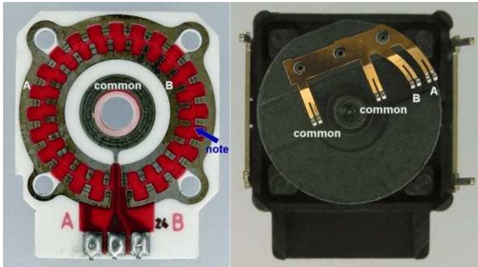
Fig. 1.6: Incremental contact encoder disc [18]
