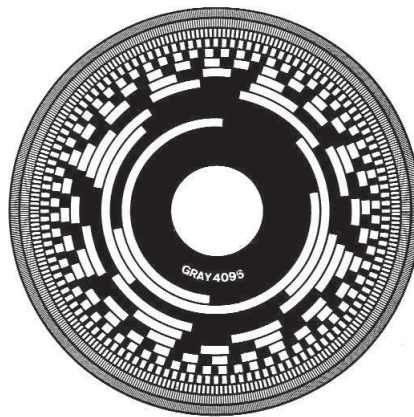
Fig. 1.9: 12bit Absolute optical encoder with gray code [22]
