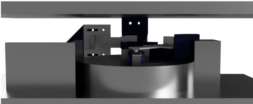
Fig. C.4: Render of platform with holders on both axes with upper optic part
