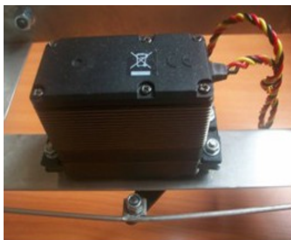
Obr.č. 7: Servomotor HS-5745 MG [4]
