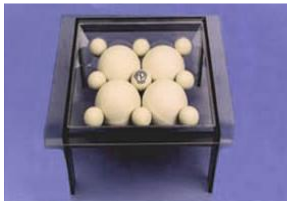
Obr. 8: Model jednoho hnízda Wheelerova dna podle firmy Akron Porcelain & Plastics Company [7]
