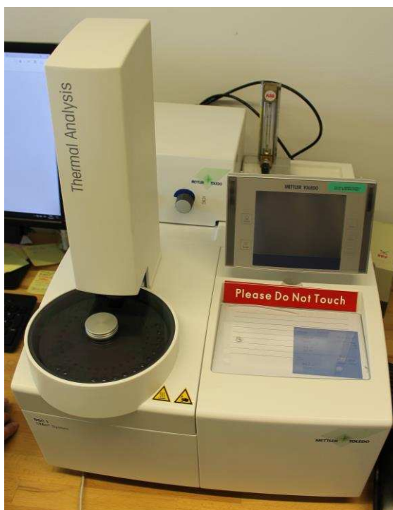
Obr. 16: Mettler Toledo DSC 1/700
