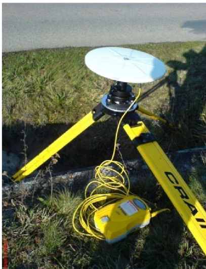
Obr. 6.1 Aparatura Trimble Zephyr nad bodem 509
