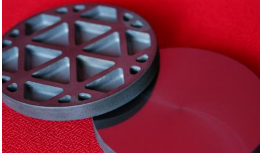
Figure 1: Example of spherical mirror from SiSiC and lightweight base plate structure [22]
