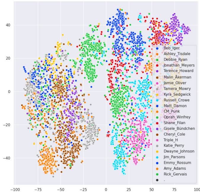
Figure 7.1: t-SNE visualization of d-vector embeddings extracted from VoxCeleb dataset. Even though there are some visible clusters, most speakers cannot be properly separated from the rest. A boundary is visible in the middle, which separates female (left) and male (right) speakers.
