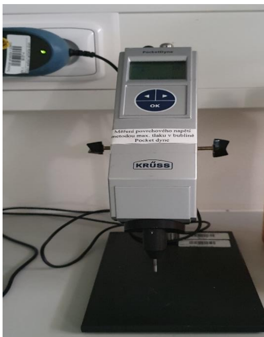
Figure 13: Surface tension measurement device.
