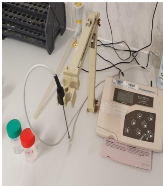
Figure 12: Conductivity testing equipment.
