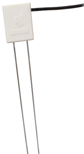
Obrázek 5: TDR senzor Campbell Scientific CS650 (Campbell, ©2022).
