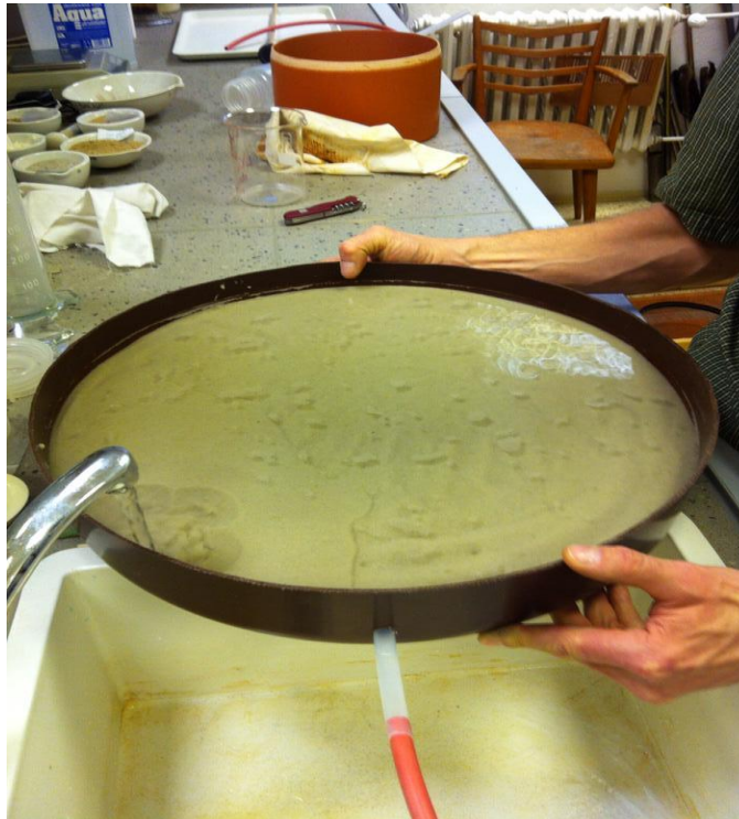
Figure 5: Homemade sandbox filled with water prepared to hold the sand sample to be examined.
