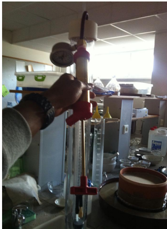
Figure 7: Filling the Guelph reservoir with water.
