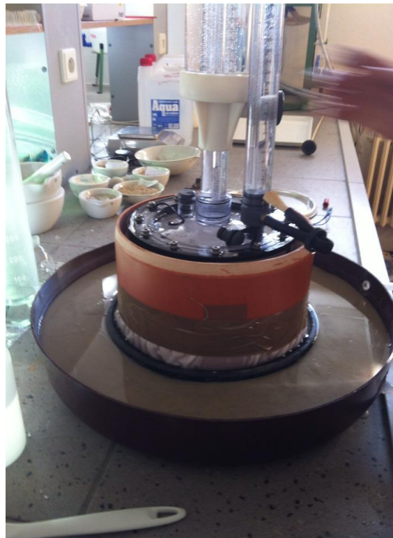
Figure 8: Guelph Permeameter on the top of the soil to initiate the process of infiltration.
