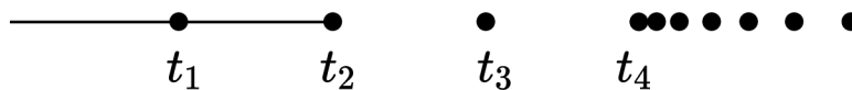
Figure 2.1: Point classification: t_1 – dense, t_2 – left-dense and right-scattered, t_3 – isolated, t_4 – left-scattered and right-dense
