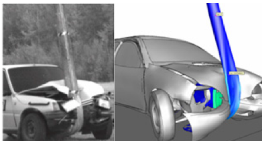
Obr. 7.10 Experiment vs. LS-DYNA simulace [13]
