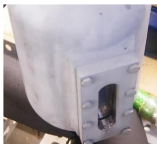
Figure 4.7 The vapor separator with a glass window
