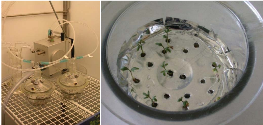
Fig. 8: Glass desiccators with artificial atmosphere placed in the growth chamber (left) and detail of garden cress plants grown at air or helox at variable ambient CO 2 concentration (right).
