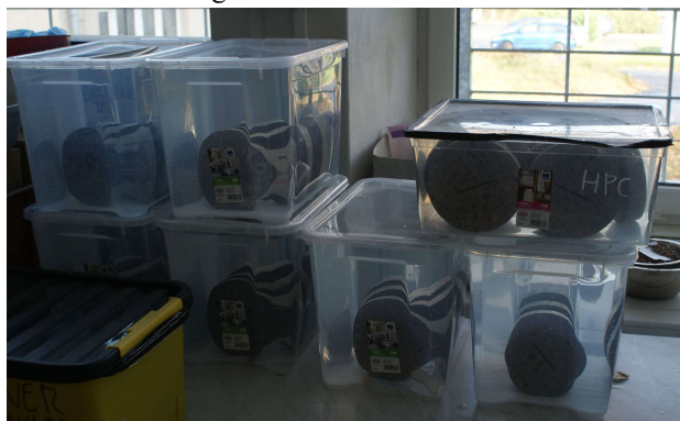
Figure 10: Prepared BD and BDCN specimens stored in plastic containers filled with water and chloride solution in a laboratory room with constant room temperature.
