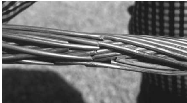
Figure 3-3 Fatigue failure of conductor strands at the suspension clamp. [2]
