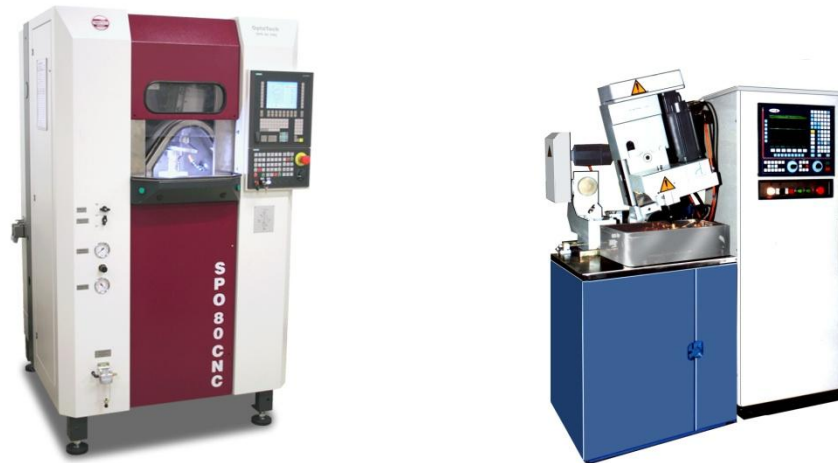
Fig. 1.3 Hybrid polishing machine "SPO 80 CNC" (left) and polishing machines for aspheric lenses "АСФЕРОИД 100П" (right)
