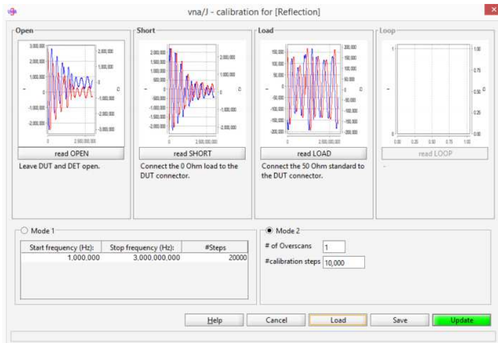
Figure 22: Calibration setup in a controlling interface of the Mini VNA Tiny
