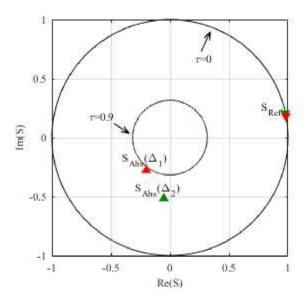
Figure 38: Constellation diagram for final values of Antenna impedances achiaved by measurement
