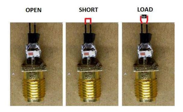
Figure 23: VNA Calibration setup
