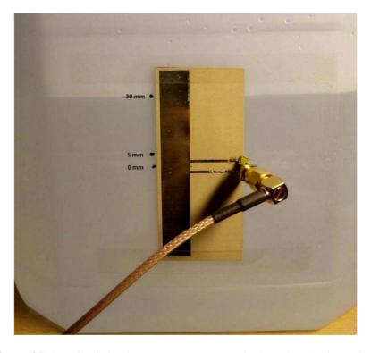
Figure 35: Detail of the Antenna prototye attached on the plastic canister
