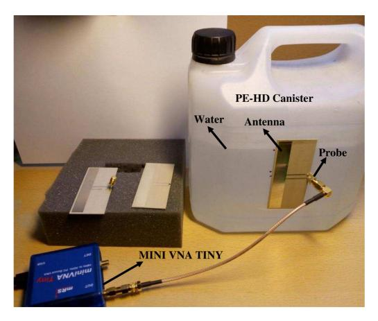
**Figure 34:** Measurement scenario including MINI VNA TINY, Plastic Canister and Tested Antenna
