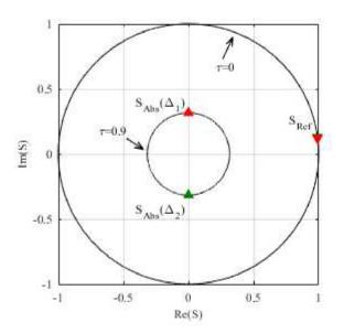
**Figure 3:** Ideal constellation diagram for 2 states: real part of absorption coefficient versus imaginary part of absorption coefficient. Two points of absorption mode (two sensing states)  $S_{Abs}(\Delta_1)$ ,  $S_{Abs}(\Delta_2)$  lie on circle  $\tau = 0.9$  and two points of reflection mode  $S_{Ref}$  lie on circle  $\tau = 0.9$
