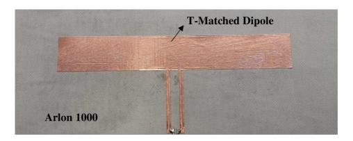
**Figure 20**: Prototype of the Antenna from a copper tape on the substrate Arlon 1000, Dimensions are corresponding to values from the Table 2.
