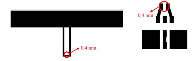
**Figure 30:** Design of the Antenna and design of the new Measure Probe with the same feeding gap
