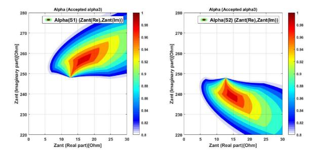
**Figure 9**: *Total efficiency α versus the* Antenna impedance.
