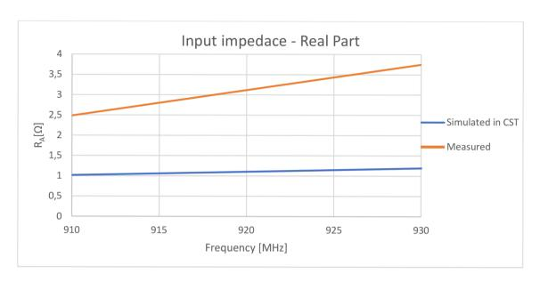
Figure 27: Input impedance of the prototype of Antenna- Real part
