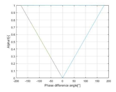
**Figure 5:** Quality of the phase modulation  $\alpha_1$  versus phase difference angle.
