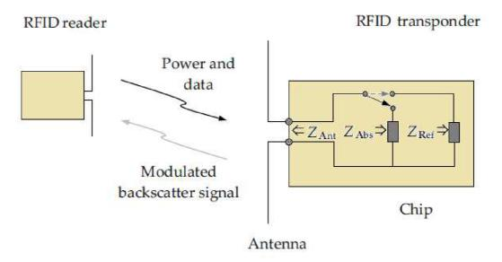
Figure 1: Principle of backscattering [1].
