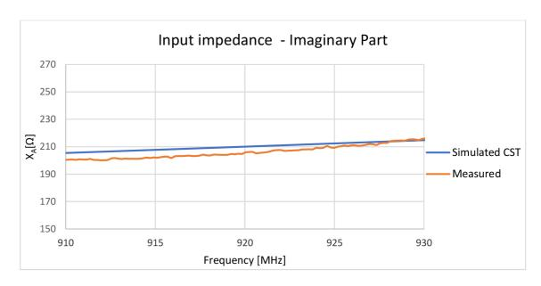
Figure 33:Input impedance of the prototype of Antenna- Imaginary part
