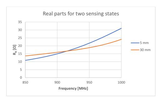
Figure 15: Real part of Antenna impedance depends on water level.
