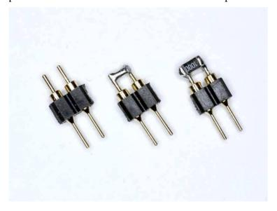
Figure 24: Realization of the Open, Short and Load situations
