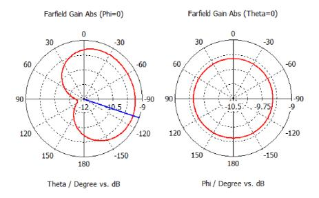
Figure 43: Simulated radiation pattern - Water 30mm, E plane (right), H plane (left
