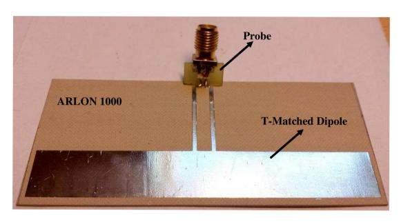
Figure 31: Seccond prototype of the Antenna with the measurement probe
