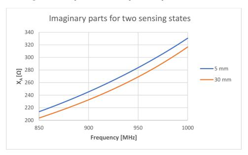
**Figure 16:** Imaginary part of Antenna impedance depends on the water level.
