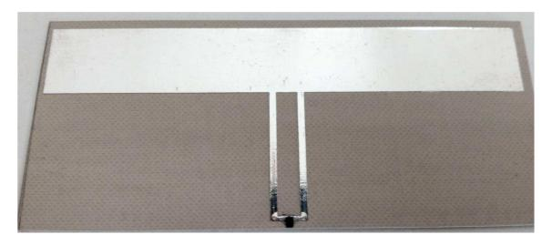
Figure 40: Final prototype with UCODE 7 chip
