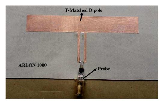
**Figure 25**: Antenna manufactured from a copper tape on a substrate Arlon 1000. Antenna board including measure Probe.
