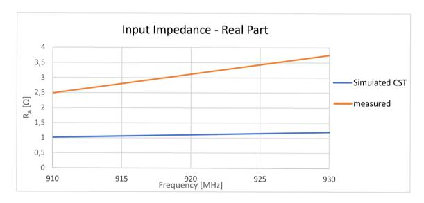
Figure 32: Input impedance of the prototype of Antenna- Real part
