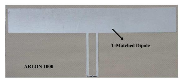
Figure 29: PCB with the Antenna Prototype which was produced by etching method
