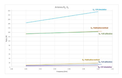
**Figure 19:** Comparison between simulated values, values provided by method from the publication and values achieved with help of full calibration of a balun
