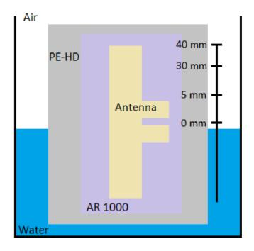
Figure 11: Scenario of level water measurement.
