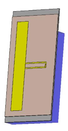
Figure 13: T-matched dipole model in CST.
