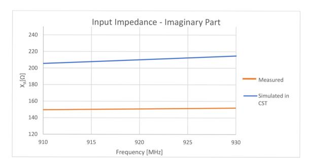
Figure 28:Input impedance of the prototype of Antenna- Imaginary part
