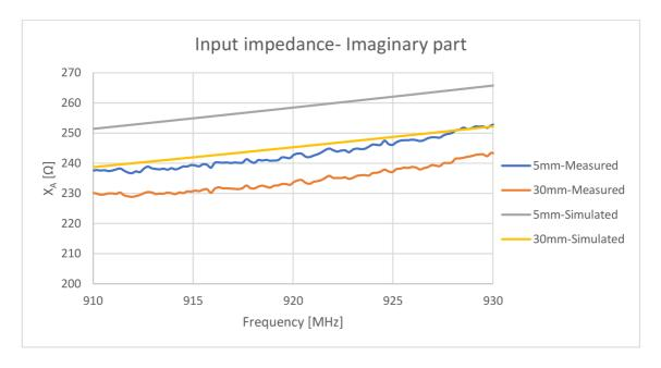
**Figure 37:** Imaginary part of impedance for two sensing states
