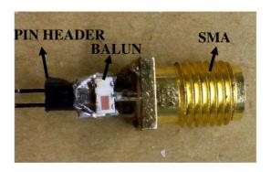
Figure 21: Measurement probe with balun including SMA connector
