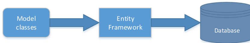
Picture 7: Generate database tables from defined model classes and context (Code First)
