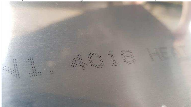
Obr. 33 Plech z oceli 1.4016 [74]
