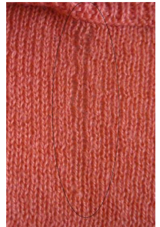
Knitting defect/ NOT OK
