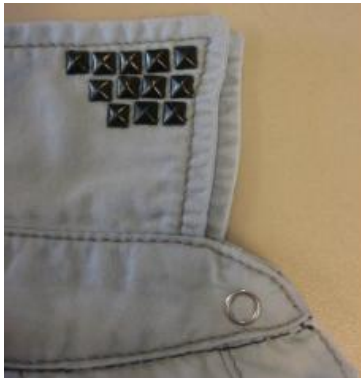
Picture 1/NOT OK ! Collar/collarband must be symmetrical
