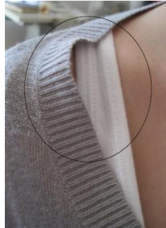
NOT OK / ribbing loosen
