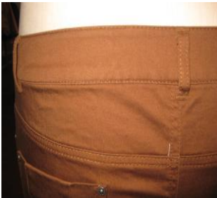
Picture 5 / Back yoke defect (excess fabric)
