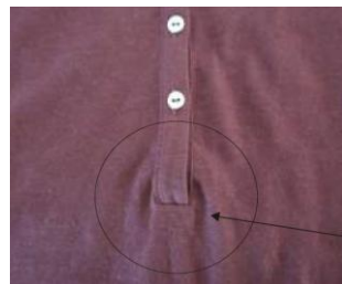
Buttontab workmanship NOT OK !
