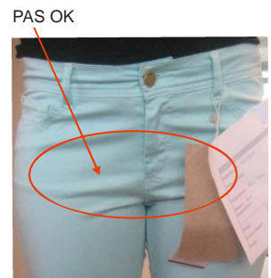
Picture 3 / Whiskers makes defect at front crotch
