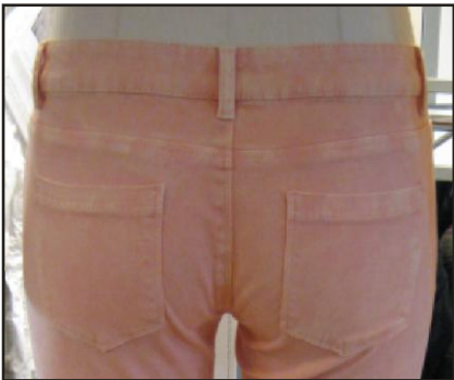
Picture 7/ Back crotch folds defect/ crotch curve not correct
