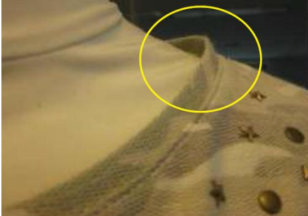
Photo 3/Do not stretch out neckline at sewing/ NOT ACCEPTABLE
