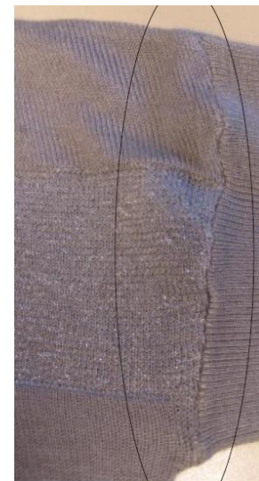
NOT OK / ASSEMBLY IS STRETCHED OUT
