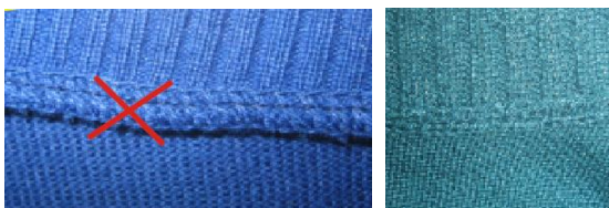
Looping assembly for neckline band.
