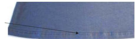
Bottom hem stretched out NOT ACCEPTABLE
