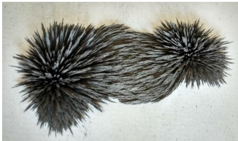
Figure 13: Magnetic field lined of a magnetic dipole depicted with help of the iron sawdust
