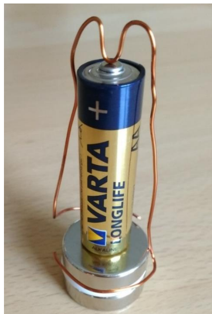
Figure 9: Realisation of homopolar motor
