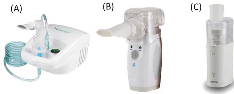
Fig. 4.2: Evaluated nebulizer devices. (A) Medisana jet nebulizer. (B) Dittman ultrasonic nebulizer. (C) Omron vibrating mesh nebulizer.
