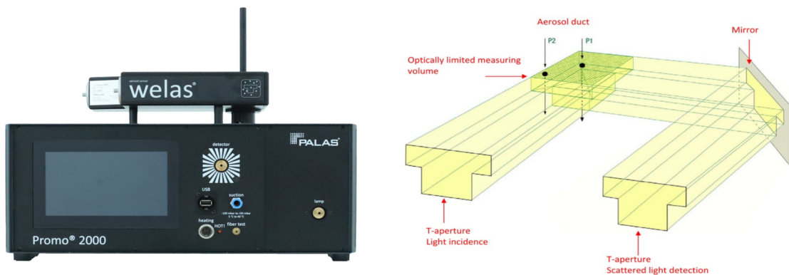
Fig. 4.6: On the left: Palas Promo 2000 spectrometer device with Welas sensor 2200 on the top and on the right: patented T-shaped aperture technology of the Promo 2000 device [48].
