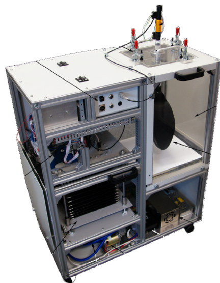
Fig. 4.4: Electromechanical Lung Simulator xPULM™ [44].
