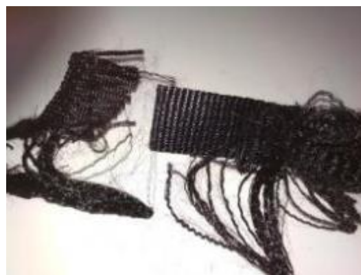
Obrázek 47 - Destructive test of strap P2 after the test, shape 3, back view
