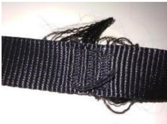
Obrázek 46 – Destructive test of strap P2 after the test, shape 3, front view
