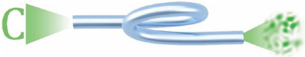
Figure 2.3: Modal dispersion and mode mixing distort the original wavefront, resulting in a complex speckle pattern at the distal end of the MMF. Figure reprinted from [39].
