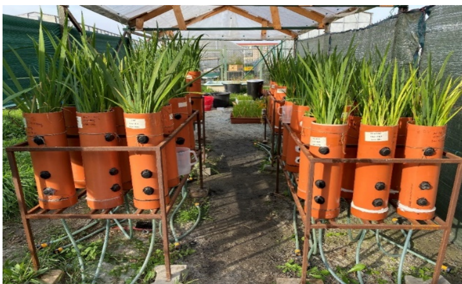
Figure 7. The vertical subsurface flows CWs simulation in the Czech University of Life Science, Prague
