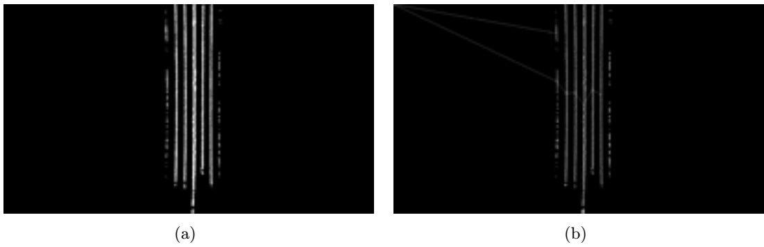
Figure 4.2: Example of the stripe indexing process. Input image can be seen on image (a). Created node tree then on image (b).
