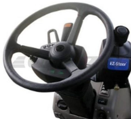
Picture 11 – EZ Steer, semi automated steering wheel by John Deere, source: John Deere
