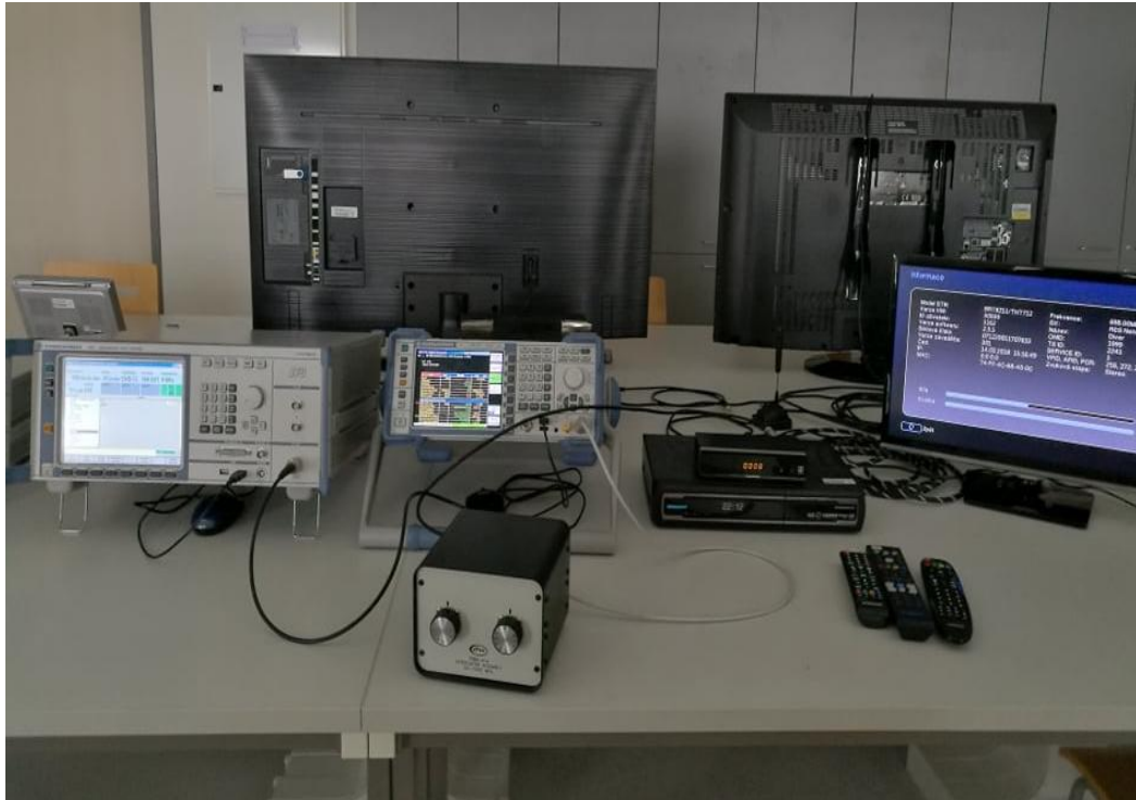
Laboratory workplace for measuring DVB-T2 performances influenced by IQ-imbalances.
