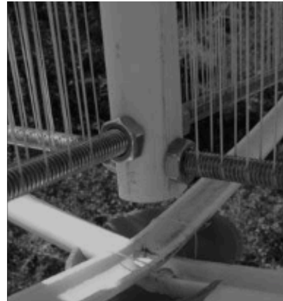
Figure 3. Actual photo of water collection device made from plastic material (PVC) of Falconer's fog collector.
