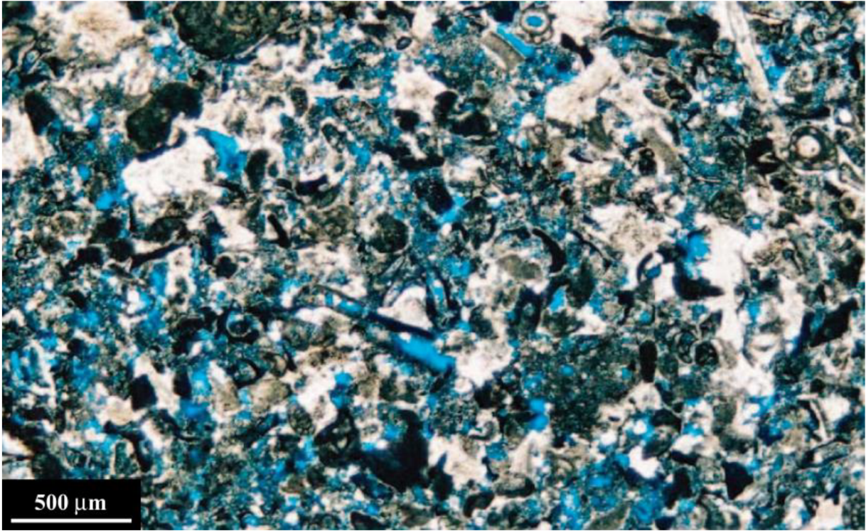
Figure 12 microporosity (10–50 \mu\text{m} pore diameter) with uniform porosity distribution, \Phi=17.6\% , k = 0.84 \text{ md} (Lønøy, 2006)
