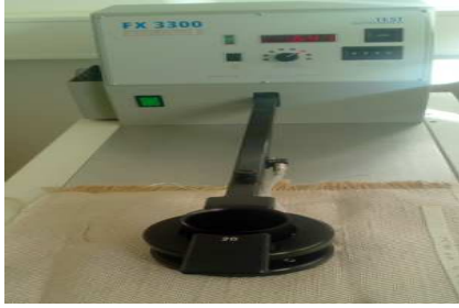
Figure 3.11: Schematic diagram of the experimental set up to measure air permeability [116]
