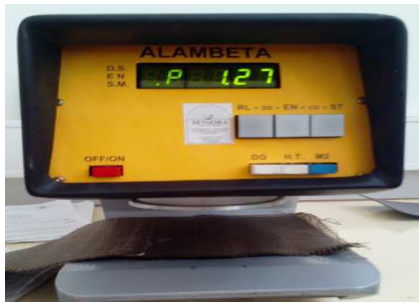
Figure 3.12: Schematic diagram of the experimental set up to measure thermal properties [115]
