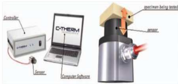
Figure 3.13: Schematic diagram of the experimental set up to measure thermal properties [117]
