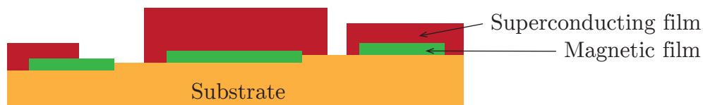
Figure 2.1: Schematic drawing of the desired superconducting-magnetic interface preparation. The magnetic film is first deposited onto the clean and atomically flat substrate. Subsequently a superconducting film is deposited partially over the magnetic film.
