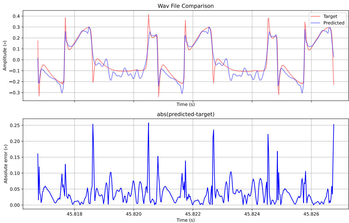
Fig. 5.4: Detailed waveform and absolute error plots of the feedforward muff model.
