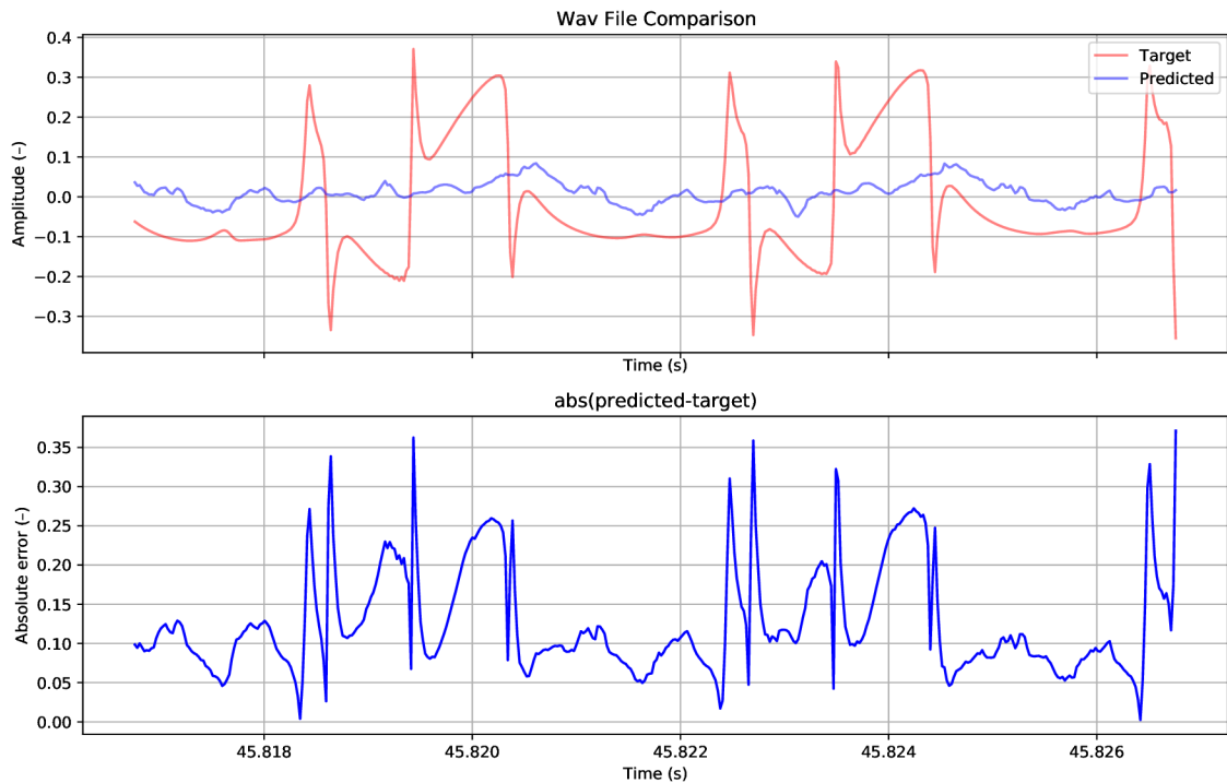
Fig. 5.5: Detailed waveform and absolute error plots of the WaveNet-style muff model.
