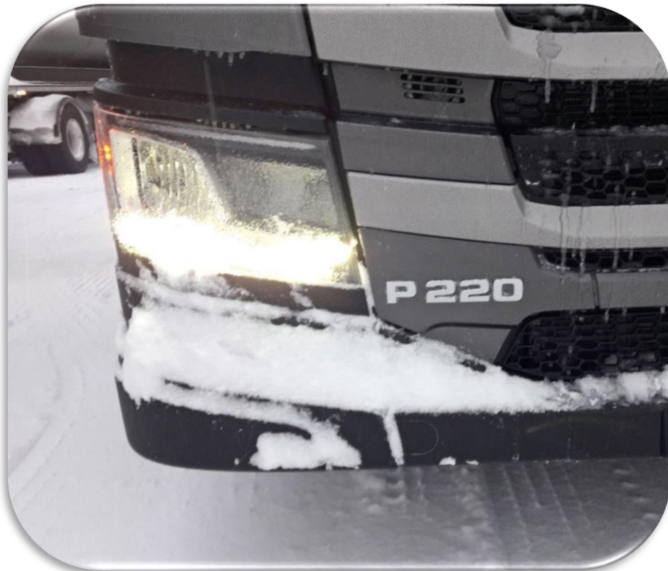
Figure 6.1. Ice layer on the headlamp cover lens [38]
