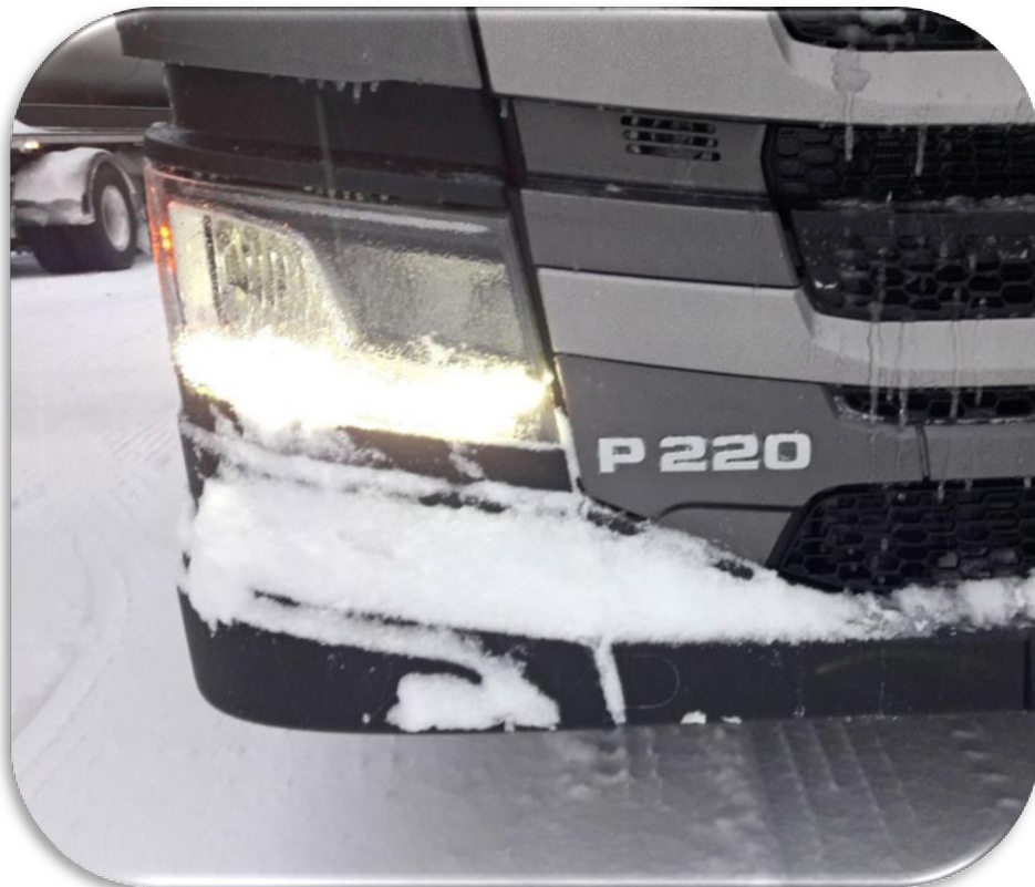
Figure 6.1. Ice layer on the headlamp cover lens [38]
