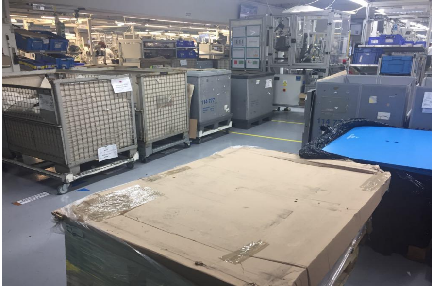
Figure 15 : Direct KANBAN boxes from warehouse (Own)
