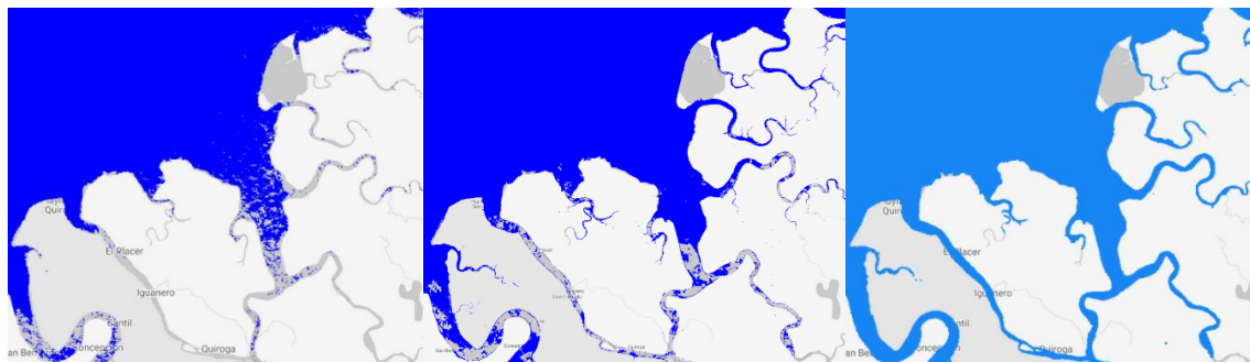
Fig 17. Comparison between Sentinel-2 water mask applied to greenest pixel composite (first image), S2 water mask applied to the median masked image (second), and Sentinel-1 water mask (third) (Google basemap)
